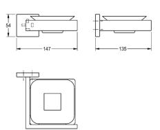
Soap dish for wall mounting, 304 stainless steel, glass dish, square covers with drilled hole on bottom for fixation, includes stainless steel screws and dowels.
