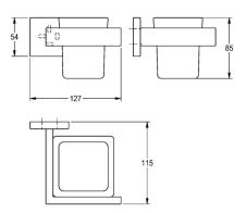
Tumbler holder for wall mounting, 304 stainless steel, square glass cup, square cup with drilled holes on bottom for fixation, includes stainless steel screws and dowels.
