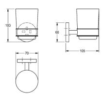
Tumbler holder for wall mounting, 304 stainless steel, glass cup, round covers with drilled hole on bottom for fixation, includes stainless steel screws and dowels.
