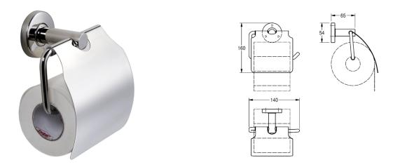
Toilet roll holder for wall mounting, 304 stainless steel, for 1 roll with max. diameter 130 mm, stainless steel folding cover, round cover to conceal the fixing of screws, includes stainless steel screws and dowels.
