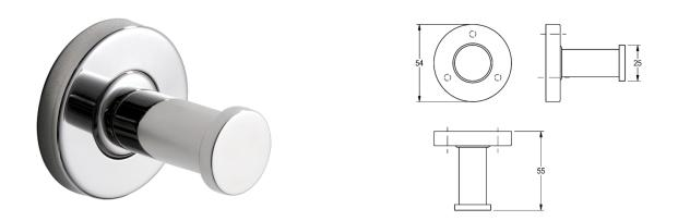
Single robe hook for wall mounting, 304 stainless steel, round cover to conceal the fixing of screws, includes stainless steel screws and dowels.
