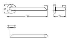
Towel arm for wall mounting, 304 stainless steel, round covers to conceal the fixing of screws, includes stainless steel screws and dowels.
