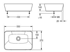
QUADROtop countertop basin, made of MIRANIT resin-bonded mineral material with pore-free, alpine white smooth surface (temperature-resistant up to 80 °C). Rectangular shape with rounded edges and seamless bowl, without overflow. No silicone sealant is required due to the invisible seal which is integrated in to the mounting edge. Drilling templates and mounting materials included.
