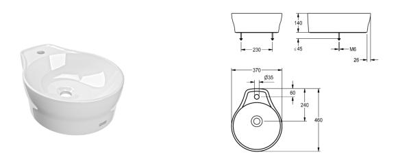
RONDAtop countertop basin, made of MIRANIT resin-bonded mineral material with pore-free, alpine white smooth surface (temperature-resistant up to 80°C). Round shape with seamless bowl, without overflow, with shaped, lowered tap ledge and 35 mm tap hole (D). No silicone sealant is required due to the invisible seal which is integrated in to the mounting edge. Drilling templates and mounting materials included.
