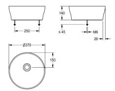
RONDAtop countertop basin, made of MIRANIT resin-bonded mineral material with pore-free, alpine white smooth surface (temperature-resistant up to 80 °C). Round shape with seamless bowl, without overflow. No silicone sealant is required due to the invisible seal which is integrated in to the mounting edge. Drilling templates and mounting materials included.
