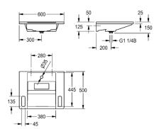
EXOS. single washbasin, wheelchair accessible, made of MIRANIT resin-bonded mineral material with pore-free, smooth gelcoat high-pol ished surface (temperature-resistant up to 80 °C). Colour Alpine white, with integrated grab rails, storage surfaces. Mounting on washbasin back panel. It has a seamless moulded bowl, no overflow and lowered tap ledge with tap hole. Mounting material, strainer waste G 1 1/4 B, anti-theft device for waster cover with InoxPlus coating included.
