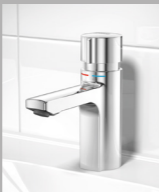
F5 self-closing pillar mixer tap For connecting to hot and cold water. 4.8 litres per minute flow rate (3 bar). F5SM1001 208.0563.593
