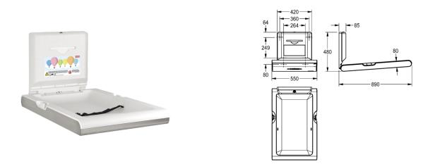
CAMBRINO vertical baby changing table for wall mounting, made of polypropylene with antibacterial Biocote® protection, white colour, front panel made of stainless steel, hinged, with integrated shock absorber for safe opening and closing, nylon safety belt and hooks on both sides, lockable dispenser for single-use paper covers in Interfold folding with maximum width 260 mm. Certified according to EN 12221-1 and EN 12221-2. Including mounting material and 80 single-use paper covers.
