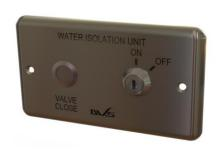
6V Isolation System, designed to shut off a water supply to a 6V latching valve. This prevents water wastage and possible overflow damage. Works via a momentary push button (to close the valve) and key switch (to isolate the power). Mains operation recommended.
