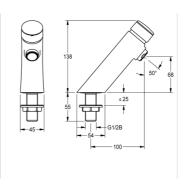
F3S Self-closing pillar tap DN 15 for sanitary facilities. Self-closing cartridge, hydraulically controlled, piston-free design, self-closing, stepless adjustment of flow duration. For connection to pre-mixed hot water or cold water. Casing, high-polished chromium-plated brass. Aerator with an integrated flow regulator 3.0 l/min.
