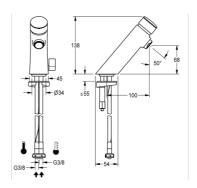
F3S-Mix self-closing pillar mixer DN 15 for sanitary facilities. Self-closing cartridge, hydraulically controlled, piston-free design, self-closing, stepless adjustment of flow duration. For connection to hot water and cold water via hoses with integrated backflow preventer and strainers. Temperature lever with adjustable, turn-proof temperature stop. Casing, high-polished chromium-plated brass. Aerator with an integrated flow regulator 3.0 l/min.
