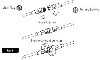
Rotate fixing against thread to lock connection
