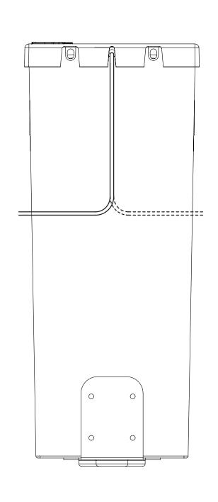
Position the base of the cistern on to the bracket fixed in the previous step, now ensure the flushvalve cable trails downwards **only** and exiting to the left or right (as above).
