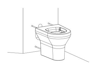
Screw the M12 studding into the back of the pan as far as possible. Make sure a flush pipe cone and outlet connector is fitted in the back of the pan. Allign the pan with fixing holes.
