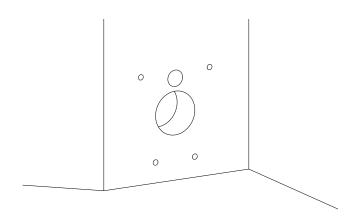
Use the drilling template provided mark and drill holes for the inlet, waste and fixing studding.
