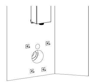
Secure the pan to the wall using the nuts and washers supplied- tighten using a torque wrench to 22-24 Nm.
