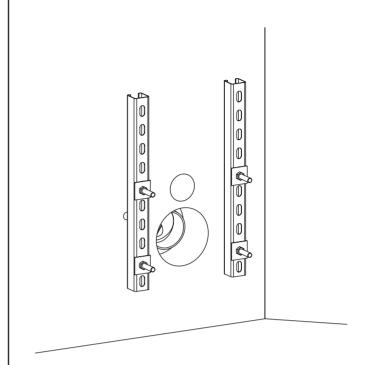
Secure the pan using the nuts and washers supplied- tighten using a torque wrench to 22-24 Nm. Connections to the WC flush pipe and soil pipes are conventional.
