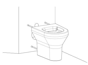
Screw the M12 studding into the back of the pan as far as possible. Make sure a flush pipe cone and outlet connector is fitted in the back of the pan. Allign the pan with fixing holes.
