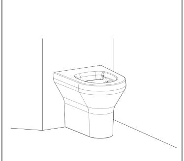
Place the pan against the wall so all the fixing studs protrude through into the service duct.
