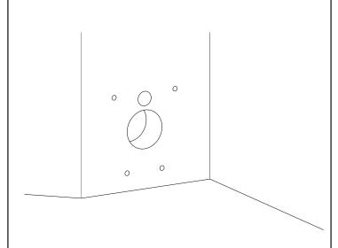
Use the drilling template provided mark and drill holes for the inlet, waste and fixing studding.
