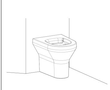
Place the pan against the wall so all the fixing studs protrude through into the service duct.
