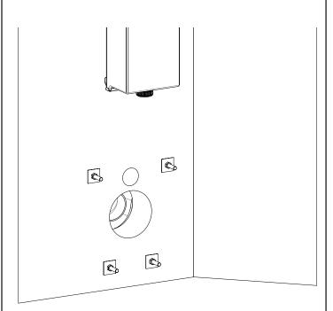
Secure the pan to the wall using the nuts and washers supplied- tighten using a torque wrench to 22-24 Nm.
