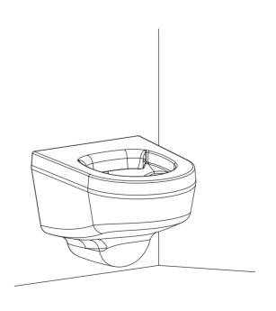
Depending on the local site requirements, anti-pick or silicone sealant can be used around the edges for finishing off.
