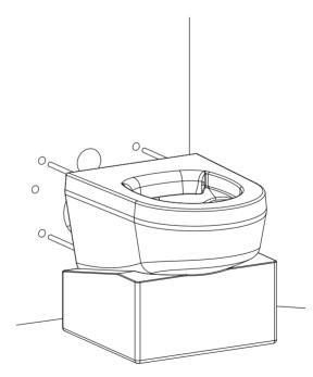
Screw the M12 studding into the back of the pan as far as possible. Make sure a flush pipe cone and outlet connector is fitted in the back of the pan. The cradle can be used to support the pan. Allign the pan with fixing holes.
