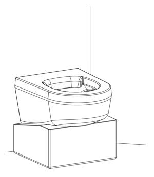
Using the cradle, slide the pan in to place against the wall so all the fixing studs protrude through in to the service duct.
